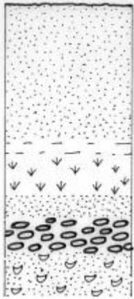
**Underlayers:** Sand on silt/clay on peat on sand on beach-worn greywacke stones (2-100mm discoid) on sand with some shells.
